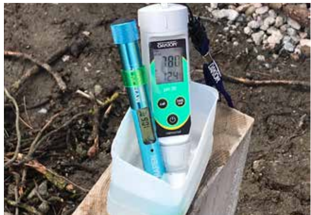
Field monitoring instruments are used to confirm water quality prior to discharge to the City's storm sewer system.
