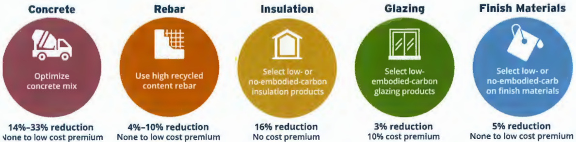
Figure 2 – This infographic, which is part of the RMI report, shows the reductions in embodied carbon and their impact on cost.
