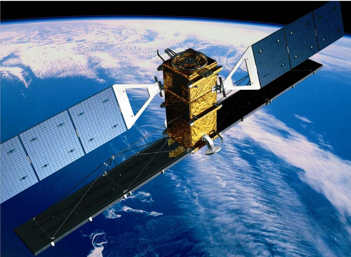
*Designed, built and operated by MacDonald, Dettwiler & Associates Ltd. (MDA), headquartered in Richmond, the RADARSAT-2 is recognized as the most capable synthetic aperture radar satellite in the world. It monitors agriculture, oceans, global climate change and disaster areas stricken by earthquakes, tsunamis and tornadoes.
