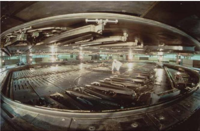
56-foot diameter TRIUMF Cyclotron: vacuum chamber and resonators built in 1969 at Ebco Industries (the parent company of Advanced Cyclotron Systems, Inc.) Photo credit: Ebco Archives/ TRIUMF.
